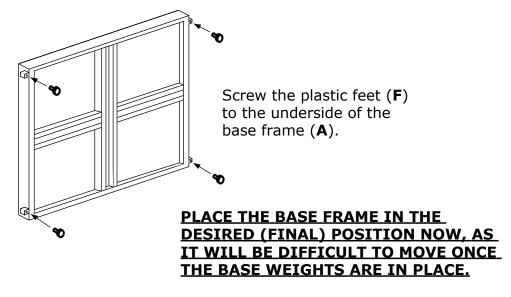
Adjust the feet to allow for uneven ground.
