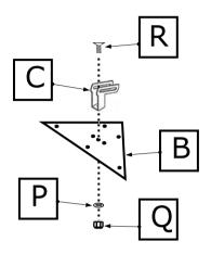
THE REMAINING 4 RIB BRACKETS-C, ARE ATTACHED TO POST BRACKETS-B, WITH M5 BOLTS-R, WASHERS-P AND NUTS-Q.
