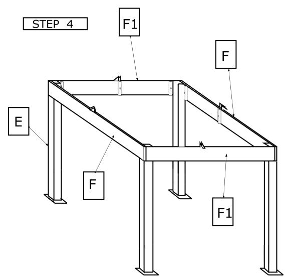
ONCE TWO END SECTIONS ARE ASSEMBLED, STAND THEM UP AND BOLT THE OTHER TWO CROSSRAILS-**F1** INTO POSITION.
